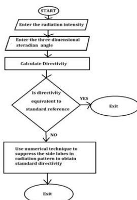
(iv) Block diagram for realizing directivity of microstrip patch antenna:-
