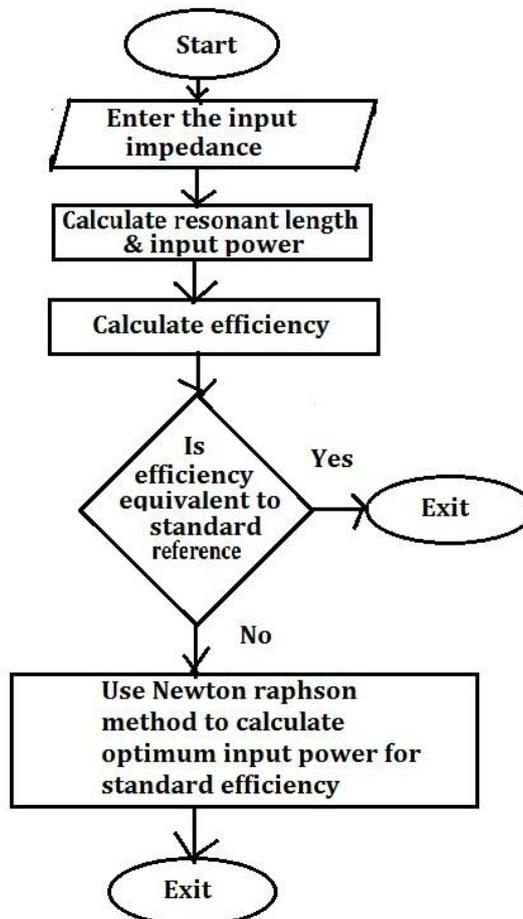
Block diagram for realizing optimum power:
